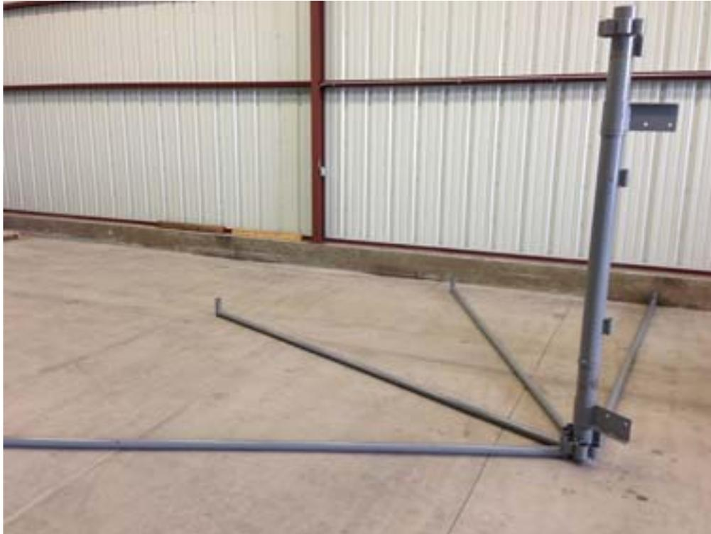
6. Place the three 7-foot uprights on the stub pipes at the end of the radial pipes with the 1/2 inch set screws at the bottom. There will be a tab at the top. There are three vertical uprights. Leave the fourth radial pipe open for the A frame. Don't tighten the set screws yet.
