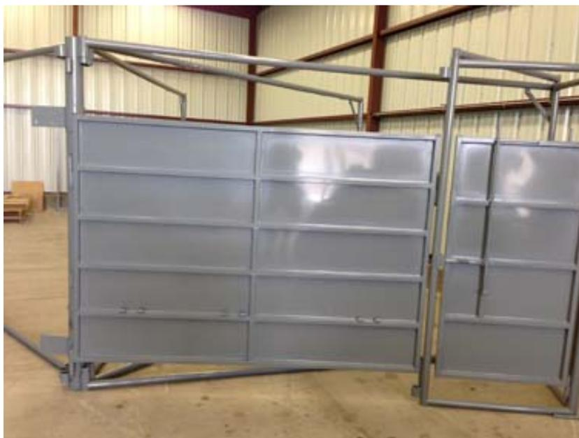
15. Start at the A frame and pin the three cleated panels to the uprights. The cleats should face the inside of the tub, toward the animals.
