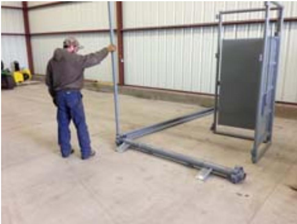
4. Pull the radial pipe that is standing vertical. This stands the pivot pipe up and puts the radial pipes on the ground.
