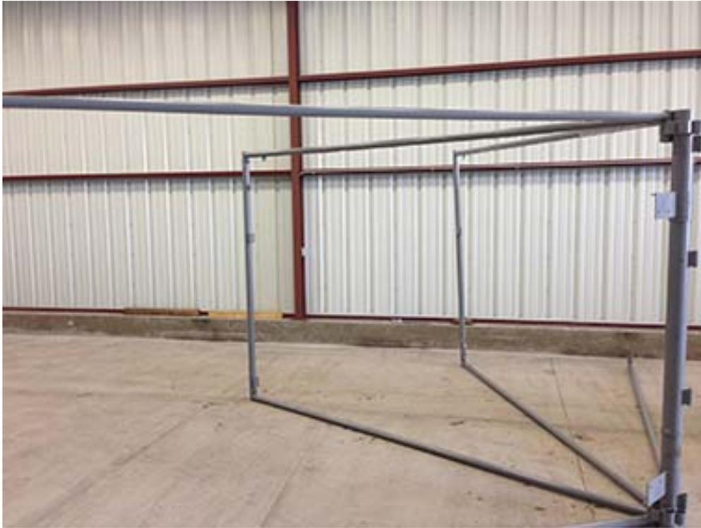
9. Install keeper bolts on both the top and bottom spreaders.
