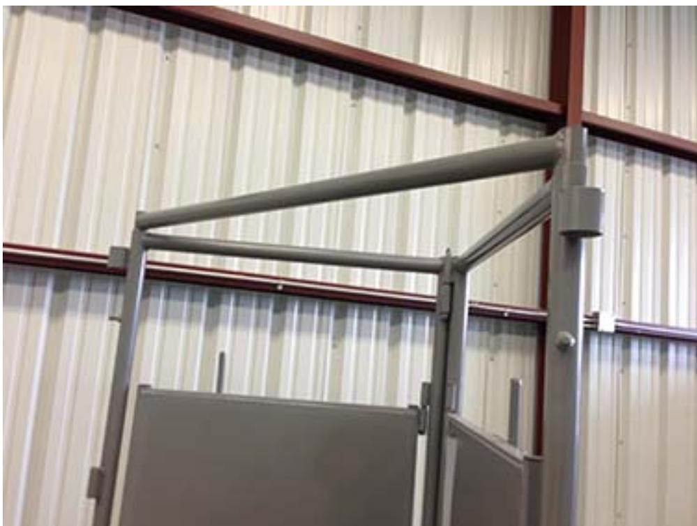
12. Place the final top radial pipe down through the collar of the pivot pipe and the end with the bolt bracket down into the top of the collar on the A frame.
